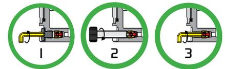
For CISO models only: remove valve from side port
