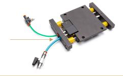
Turn and lift the scrap remover, let the (filtered) air at 6-8 BAR into the scrap remover for 1 min. to blow dirt out. **Warning: mind your hands!**
